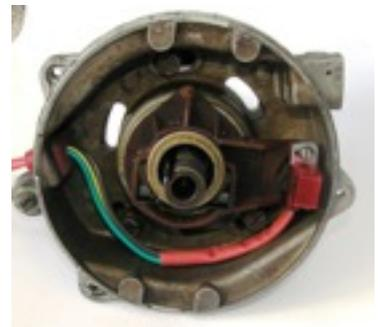
**Next install the “REOPUS H” circuit board into your OPUS amplifier casing.**
